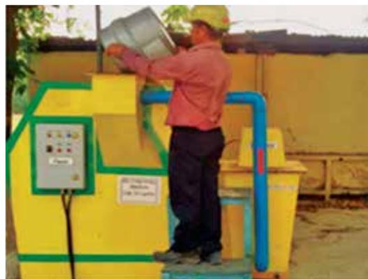
Biocompost Machine (Organic Waste to Fertilizer) at Bawal Plant
